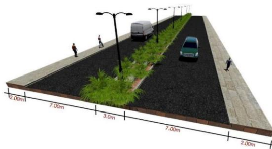
Figure 20:3 Typical Section of 21m Wide Road
