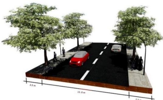
Figure 20:2 Typical Section of 18 m Wide Road
