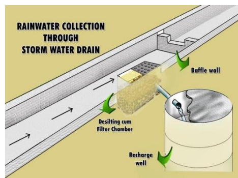
Figure 21:22 Storm water collection to recharge wells
